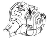
Hold the body of the machine on the ground using your left hand (CAUTION! Not with your foot!).
